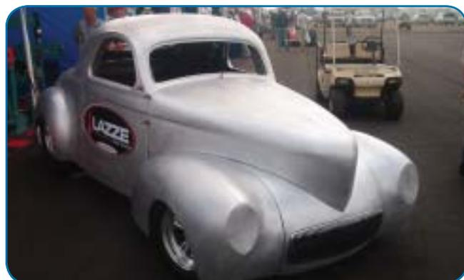
Believe it or not, this body is a completely fabricated steel '41 Willys coupe. It's a display piece for the Lazze line of metalworking tools and shop courses.
