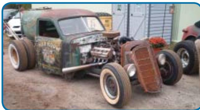
Take one well used '47 Studebaker truck cab, add an early Chrysler hemi up front, mount a tank off an ancient orchard spray rig out back and the result is a striking "rat rod" dually with lots of attention getting potential.
