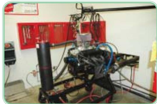
*The mild small block Chevy produced 353 horsepower at 5,500 RPM on the Van Buren Technology Center's dyno.*
