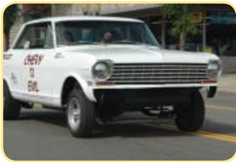
Big and little tires, straight axle, nose high attitude and no front bumper...all signs of a "bad" street/strip Nova.
