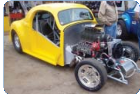
Ultra modern Willys, but check out the engine... it's a high tech Ford flathead.
