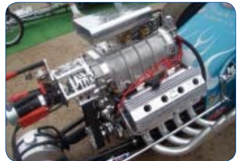
A 276 cubic inch DeSoto hemi powered the Schrank Brothers vintage fueler.
